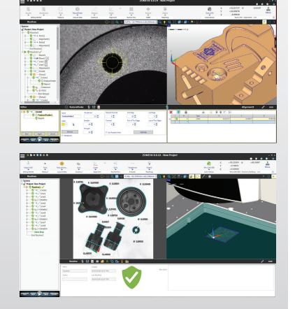
ZONE3 Prime and Pro offer extended capabilities such as 3D CAD programming and run time optimizer to measure multiple parts fast and efficiently. Parts are automatically identified and features are instantly measured to help eliminate complex programming steps.
